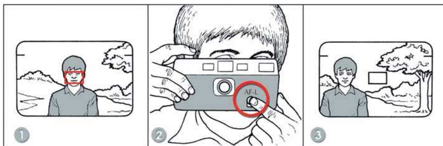
Figure 13.3 An auto-focus camera with AF lock allows you to sharply focus a main subject you compose off-center. (1) First, center the subject in the auto-focus rectangle. (2) Half depress the shutter release to make the lens focus, then operate the AF-L control. (3) Now you can compose the subject anywhere within the frame before shooting.
